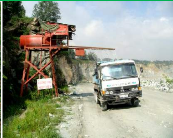
Watering stone before carrying stone out of the mining area, to avoid dust on the road transport
